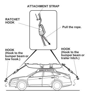
13. To loosen the rope, push up on the ratchet strap lever, then pull the rope.
