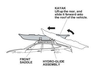
4. Adjust the distance of the saddles and hydro-glide assemblies to the same width as the kayak, then secure the saddles and the hydro-glide assemblies by tightening the knobs you installed in steps 1 and 2.
