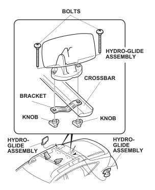
3. Rest the front of the kayak on the hydro-glide assemblies. Standing behind or alongside the kayak, lift up the rear portion of the kayak and push it forward, sliding on the hydro-glide assemblies and saddles. Make sure the kayak reaches the front saddles before you lower it.
